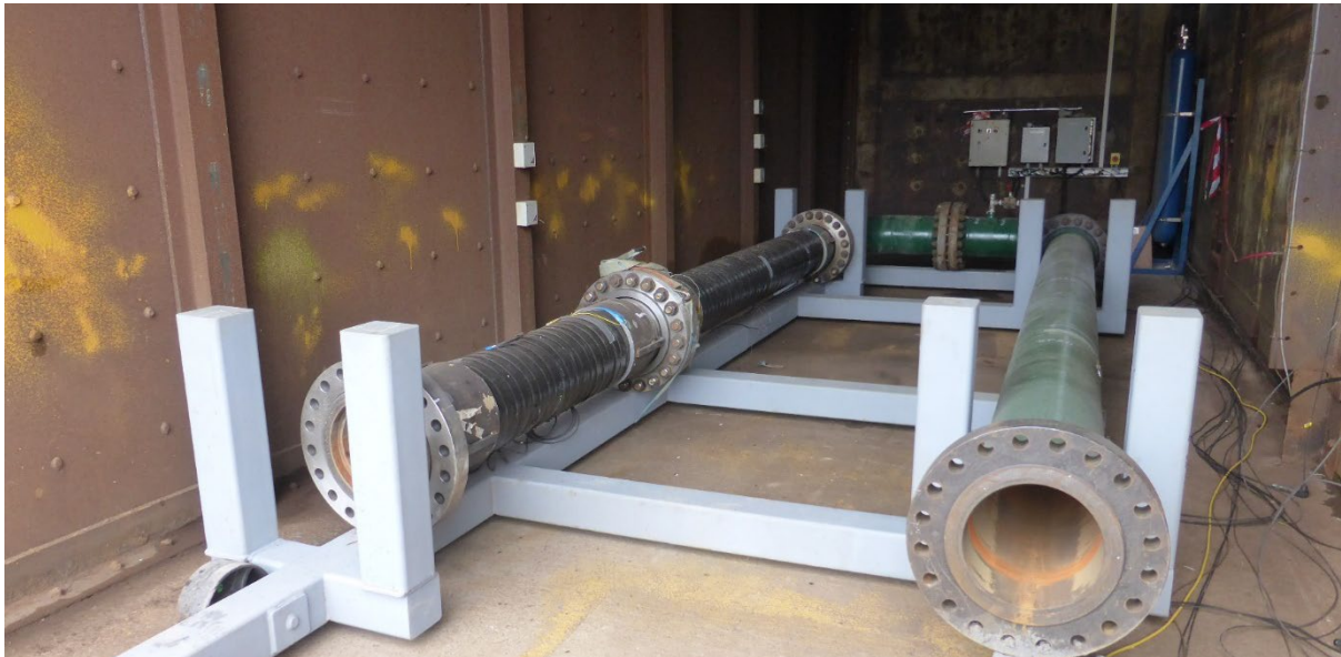
Figure 5.2 Photograph of 12 inch test pipes in test loop (a) standard X52 on the right and (b) MASiP on the left
