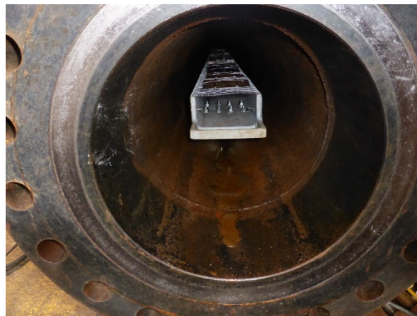
Figure 5-4 Standard test coupon tray inside pipe
